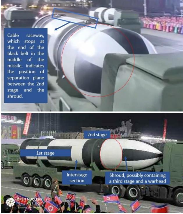
Figure 5. The cable raceway is indicative of the length of each stage of the unnamed SLBM because the cables could not be placed inside the propellant. The shroud seems to have enough length and volume to accommodate a third stage and the warhead. Images: KCTV [12], Rodong Sinmun [13]
