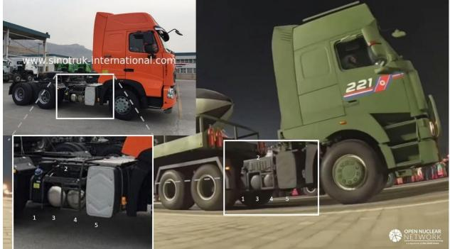
Figure 12. The accessories of the trucks seen in the parades are identical to that of the HOWO T7H commercial trucks. The truck cabins seen in DPRK parades have been modified. Images: KCTV [37], Sinotruck [38]
