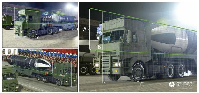
Figure 1. Example measurement of the diameter (marked as A) of the Pukguksong- $4 \checkmark$  (top left), the Pukguksong-5 (bottom left) and the unnamed SLBM (right), using the approximate height of the truck (B) and the diameter of the wheel (C) as references. The grid shows the vertical plane on which the measurement was made. Images: Rodong Sinmun [1]
