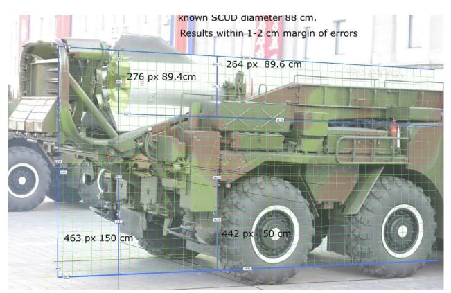
Figure 11. The SCUD missile is known to have a diameter of 88 cm. The error margin of this measurement is ~1.5 cm. The grid is a vertical plane where the measurement is made. The reference is the wheel diameter of the MAZ-543 truck. Image: Tianran Xu
