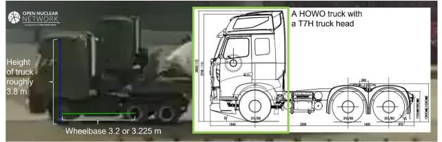
Figure 13. Height of the trucks towing the SLBMs. Inset image: dimension of a T7H truck head. Images: KCTV [40], Sinotruk [41]
