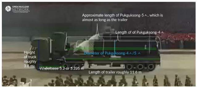
Figure 3. A rough measurement of the length of the Pukguksong-4  $\land$  and the Pukguksong-5  $\land$ . Due to the limited availability of images, a more precise measurement could not be made. Image: KCTV [3]
